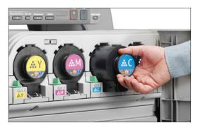
The Trained Customer Replaceable Unit (TCRU) kit includes a wide range of userreplaceable parts for convenient in-house maintenance that reduces expenses and maximizes system uptime.
