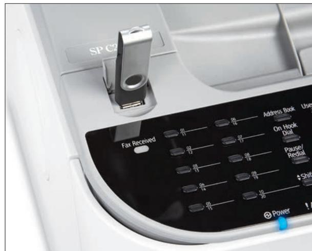
*Convenient placement of a USB port on the front of the device allows users to leverage the PictBridge interface and access the Scan-to-USB feature without a PC.*
