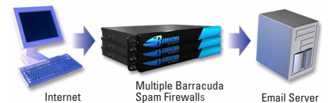
Clustering provides for redundancy and even greater capacity
