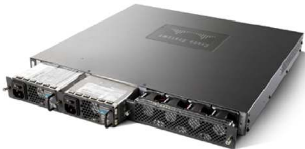
Figure 2. Rear View of Cisco Catalyst 4948 with Dual Redundant Power Supplies and Removable Fan Tray
